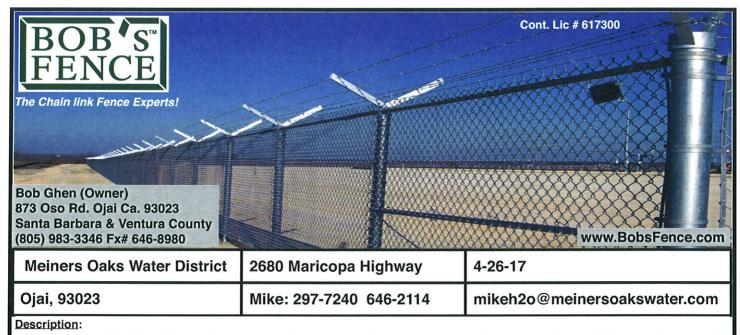
Install 716' of 6' tall 9 ga. galvanized chain link fencing with three strand 4 point barbwire. To use 2 7/8 terminal post and 2 3/8 line post set in concrete. (Concrete mixed in wheel barrel before setting, no pouring dry concrete in hole then adding water). Fence to have 1 5/8 diagonal bracing and and 9 Ga. tension wire along top and bottom. Removal of existing fence included if needed.
