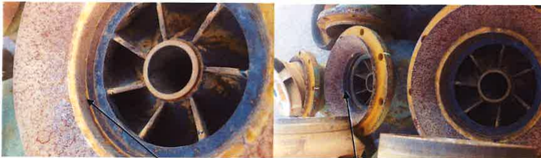
Notice Step in wear ring from wear
